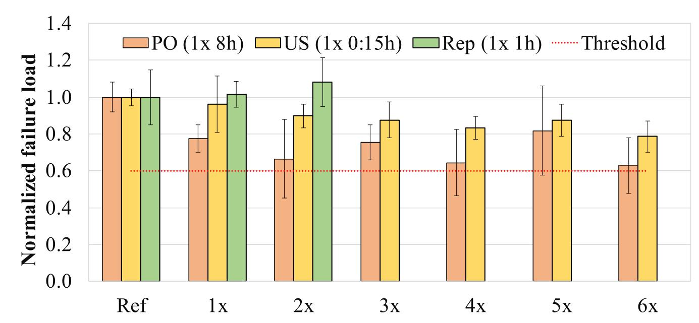
Figure 4 – Normalized shear strength of RJS joints cyclicly aged [2].
