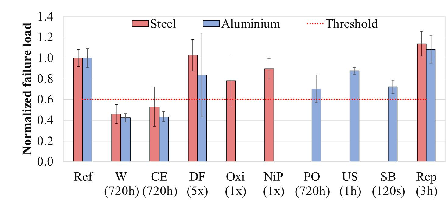
Figure 3 - Normalized shear strength of RJS joints continuously aged [2].
